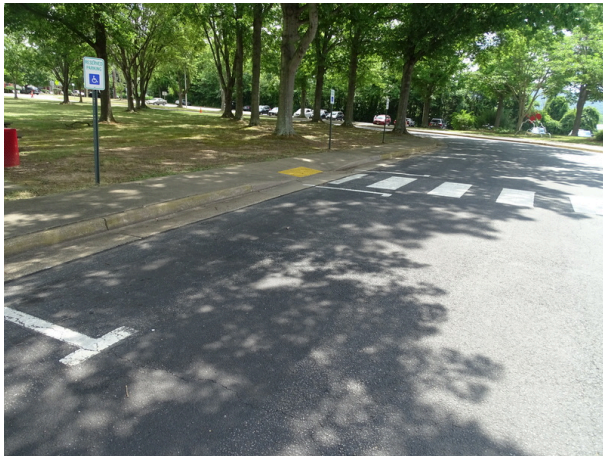
Accessible parking spaces - note only two of five needed spaces provided
